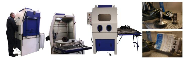
High pressure cleaning in a closed system, fast, efficient and environmentally friendly. The used cleaning liquid is reused through the continious filtration. For the cleaning and blow drying of metal and plastic parts. The complete cleaning is done manually.
